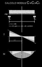
**SCHEMA STATICO E ANALISI DEI CARICHI: mod. a6-a7/a8**
