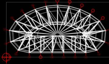
**SCHEMA STATICO E ANALISI DEI CARICHI: mod. c1-c3-c5**
